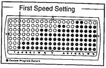
(The incline settings are not shown in the LED matrix.) The two columns on the left side of the LED matrix will be dark. The first speed setting of the program will be shown in the third column (see the drawing above); the next seventeen speed settings are shown in the seventeen columns to the right.
